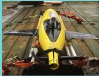
We equipped a SeagliderTM deployment with a JASCO AMAR G4 hydrophone. The glider was deployed in May 2019 and was operational for a period of 2 weeks.
